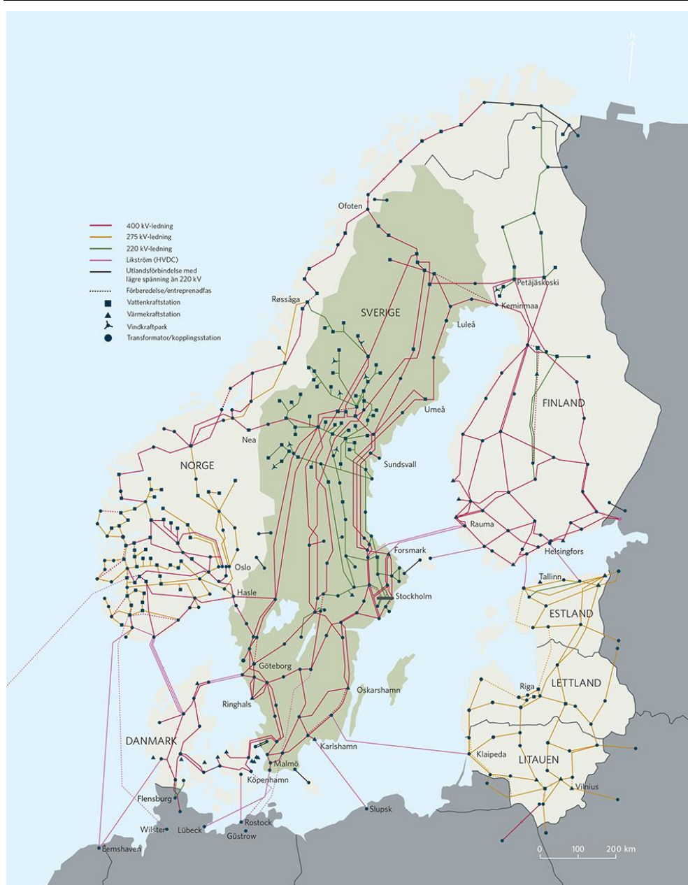
Figure 1 The Swedish transmission network for electricity and other connections to other countries
